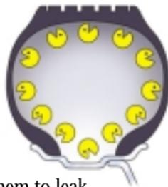
Rust and dust from wheels can clog valve stems, causing them to leak. And, rough surfaces on wheel flanges and tire beads may not seal properly, causing additional leaks.
