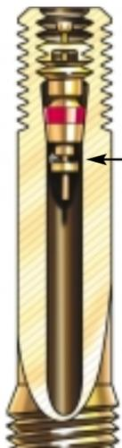
Small bits of corrosion from wheels can prevent valves from seating properly, leading to loss of air pressure.
